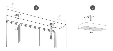
If you have a wide shade, you will need to install extra brackets to support it. These are included. Space the additional brackets equally along the width of the window opening, level with the end brackets.
