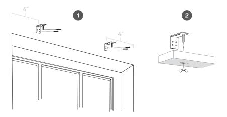
If you have a wide shade, you will need to install extra brackets to support it. These are included. Space the additional brackets equally along the width of the window opening, level with the end brackets.
