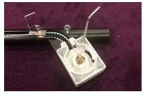
12. Spray both pulleys, interior of rail, and masters with Forest dry silicone spray. Spray lubricant on paper towel or clean soft cloth and wipe inner edge of rail.
