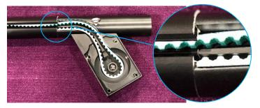
10. Once marked, pull idler side out and up, and then pull belt from motor side to reveal mark on belt. Attach belt connector and master on the mark. Carriers are added next.
